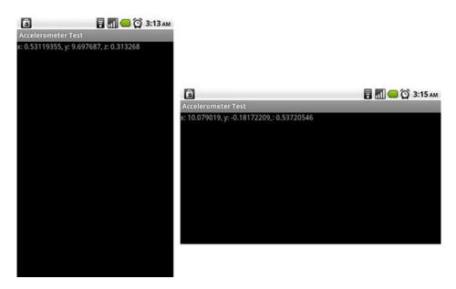
Figure 4-9. Accelerometer axes values in portrait mode (left) and landscape mode (right) when the device is held perpendicular to the ground
